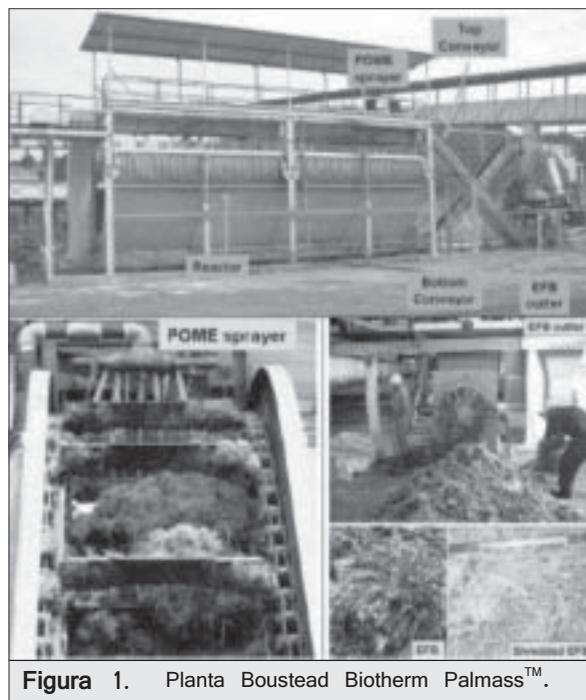
Figura 1. Planta Boustead Biotherm Palmass™.
